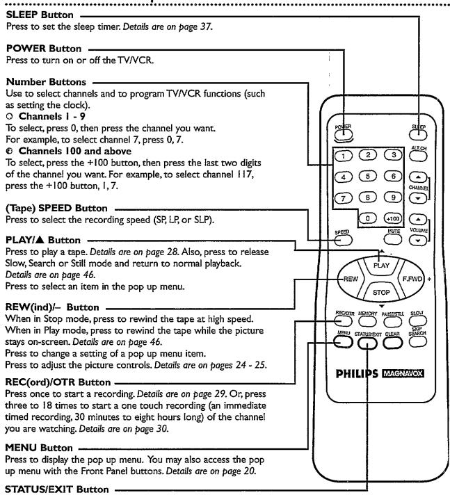
Press to see the status display. Press again to remove the status display. Details are on page 26.
